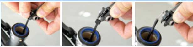
Figure 153: Removing the Bowden cable
