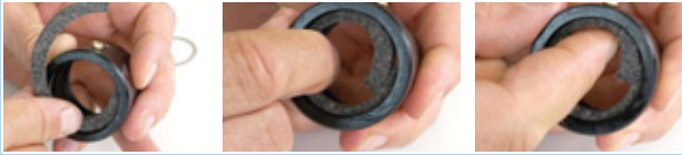
Figure 125: Inserting the felt ring
