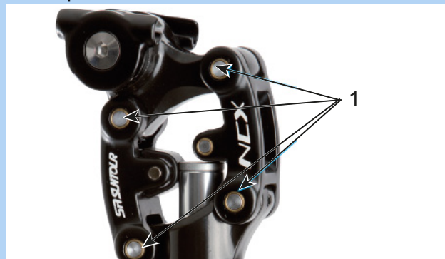
Figure 111: SR Suntour suspension seat post lubrication points
