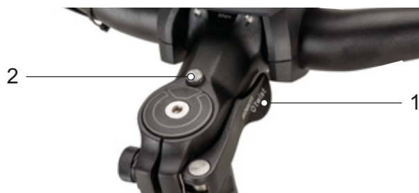
Figure 87: Stem, version II with clamping lever on the stem quick release (1) and unlocking knob (2)
