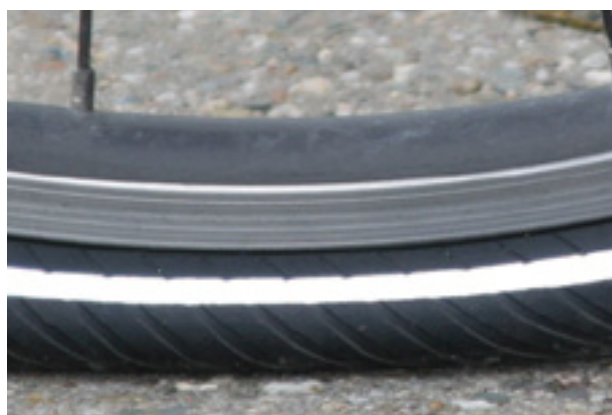
Figure 63: Much too little tyre pressure
