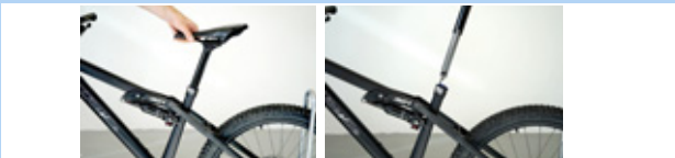
Figure 152: Removing the seat post
