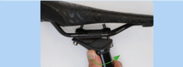
Figure 163: Opening the height adjustment
