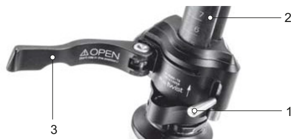
Figure 86: Opened clamping lever on the stem quick release (3) on the stem (2), version I, with locking lever on the stem (1)
