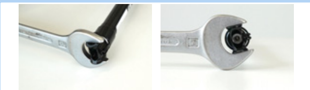
Figure 133: Securing against twisting
