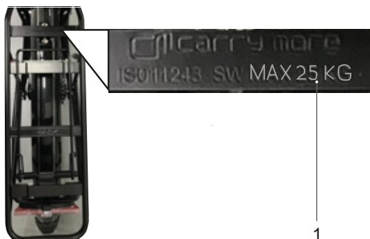
Figure 78: The maximum load bearing (1) capacity is indicated on the pannier rack.
